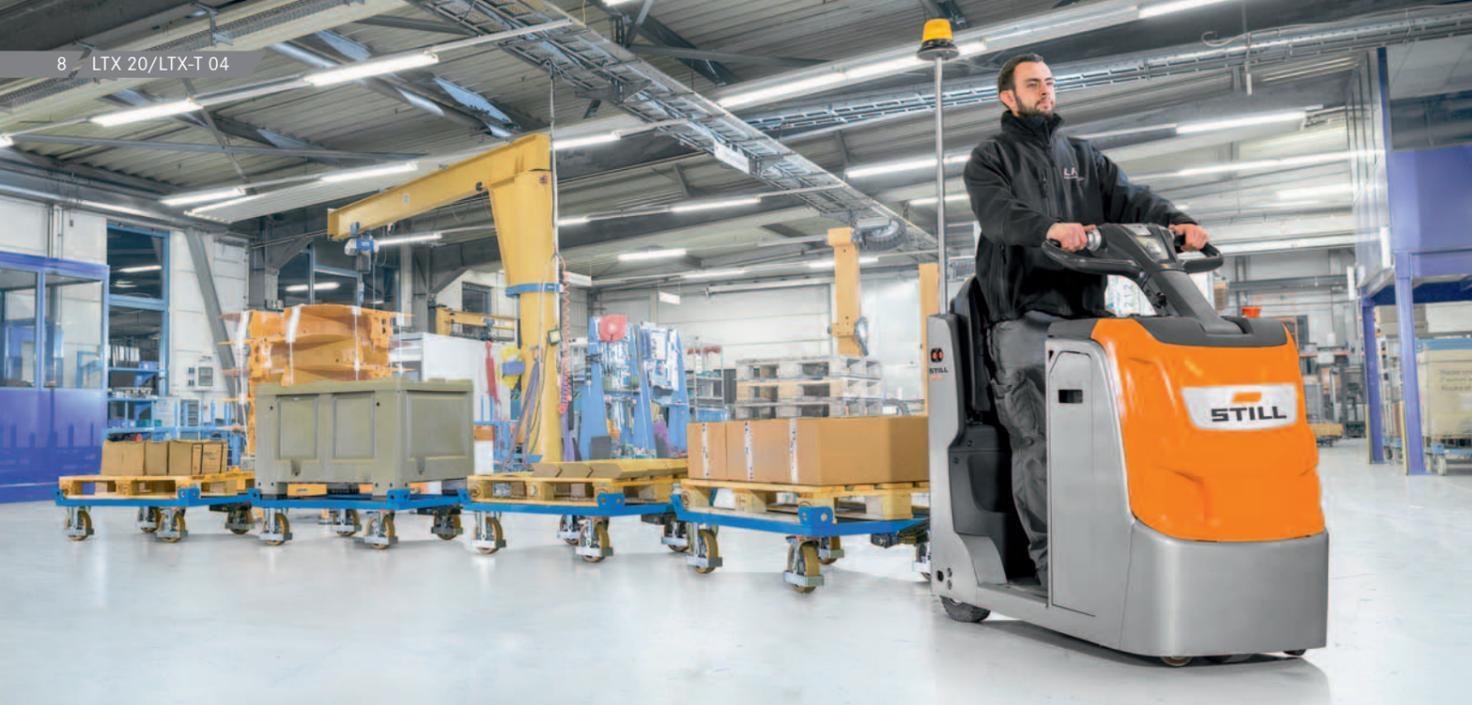
**LTX 20 und LTX-T 04.** With a slender vehicle width measuring a mere 600 mm, they are flexible and compact, even in the tightest of spaces, as well as comfortable for drivers to work in thanks to their low access step and spacious footwell - LTX-T 04 and LTX 20, multifunctional vehicles available as tractor or platform truck. An ergonomic backrest with integrated folding seat and a sprung and cushioned driver's cab make driving comfortable and efficient.
