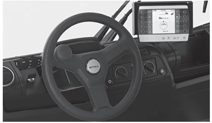
The smooth-running steering wheel with knob ensures top ergonomics. The operator also has an overview of all the available information on a large display
