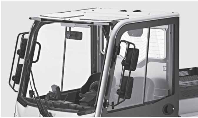
The optional STILL Flashlight, securely installed below the roof, provides a warning for people in front of and behind the truck
