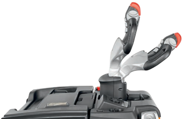
The flexibly adjustable working angle of 83° enables an ergonomic working posture of the tiller - and that for operators of any height
