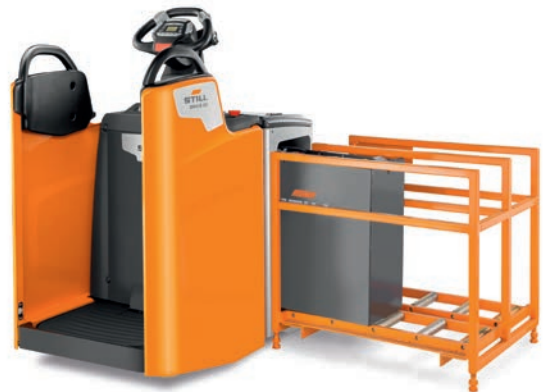
Maximum vehicle availability through lateral battery change or lithium-ion technology suitable for interim charging
