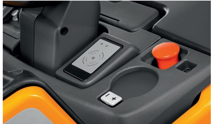
A variety of access options and a stand-on platform cushioning that can be adjusted by rocker switch (+/-)
